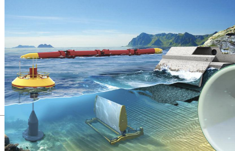
▲ Concepts for utilising wave power: Floating bodies, buoys, oscillating shutters or tidal power plants.
