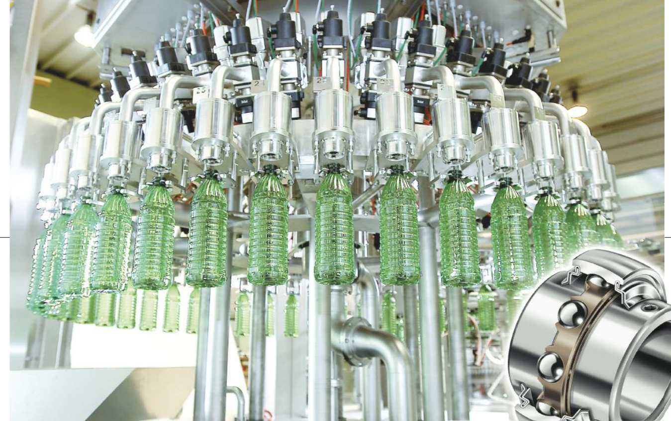
▲ The high performance capacity of slewing rings is required in product fillers for PET (Polyethylene Terephthalate) bottles
